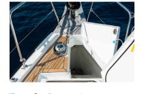
The reefing lines coming down from the boom and the halyards coming from the mast, together with the sheets of the mainsail circuit, are immediately concealed under the cowling in order to keep the deckhouse clear
